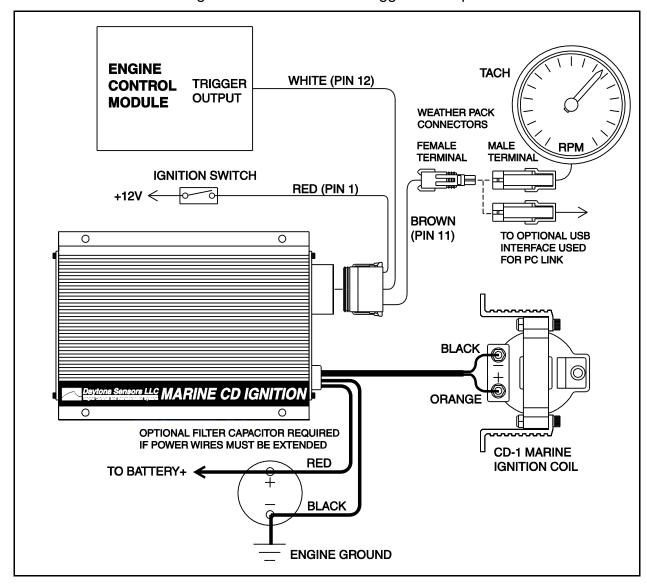
Figure 4 – Basic Module Trigger Hookup
