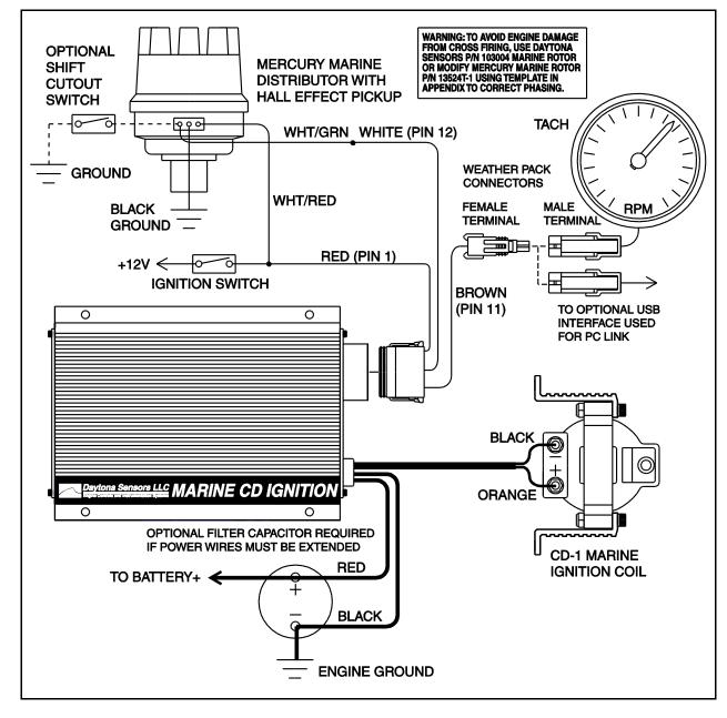
Figure 3 – Basic Mercury Marine Hall Effect Distributor Hookup
