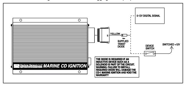
Figure 9 – GPIO3 Data Logging Hookup Options
