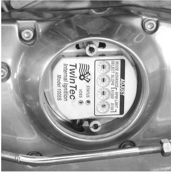
Figure 3B - Finished Sportster® Installation
