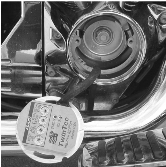
Figure 1 - Feeding Harness Thru Exit Hole
