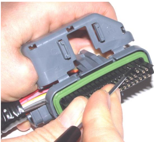
Figure 4 – ECM Connector Terminal Removal
