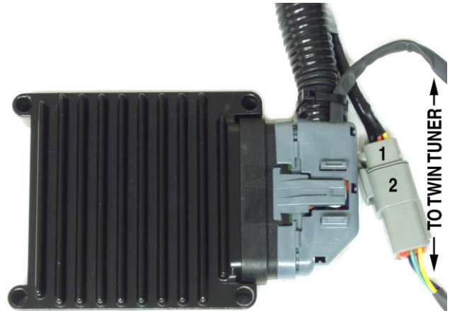
Figure 5 – Completed Wiring at ECM
