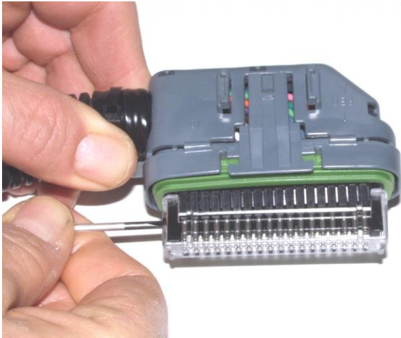
Figure 3 – ECM Connector Disassembly
