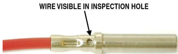
Figure 3 – Correctly Crimped Terminal
