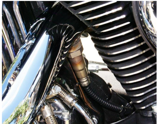
Figure 25 – Typical Rear Sensor Installation
