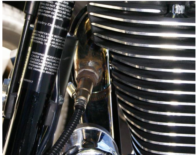
Figure 25 – Typical Rear Sensor Installation
