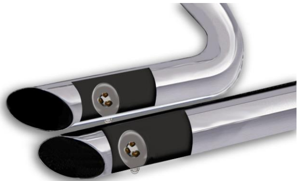
Figure 1 – Exhaust Mod to Reduce Reversion
