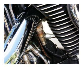
7. Connect the Bosch sensors to the 6 pin mating connectors on the WEGO wire harness. The longer cable (with yellow band) is for sensor 1 (front). For additional protection and improved cosmetics, use Techflex 1-1/4" Black Flexo Clean Cut FR expandable sleeving over the connectors (available from www.wirecare.com).
