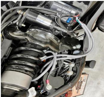
4. Do not reconnect the battery ground cable until you have completed installation of the WEGO IIID. Do not attempt to start the engine until you have completed the initial setup.
