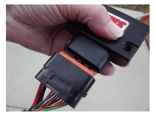
Step 2 - Locate the pedal position sensor assembly. The connector for the pedal position sensor is typically located near the top of the accelerator pedal.
