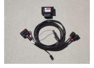
PedalMAX mounts inside the vehicle cabin, under the dash near the accelerator pedal sensor.
