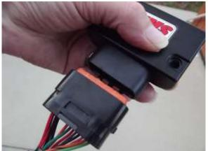
**Step 2 - Important:** Disconnect the positive terminal of the battery before installing this product. If you do not disconnect the battery the factory computer will not learn the correct starting pedal position.
